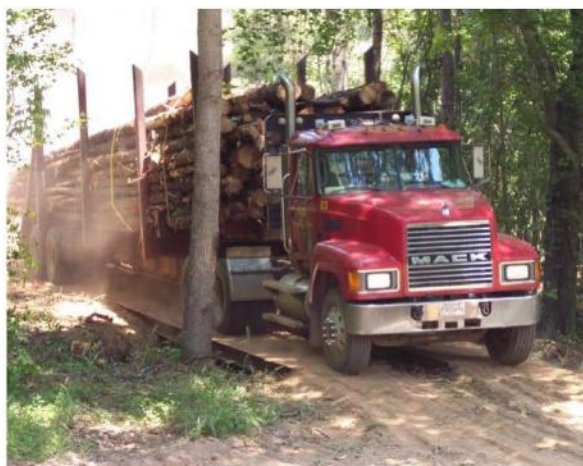
Log truck utilizes a temporary steel bridge to cross a perennial stream.
